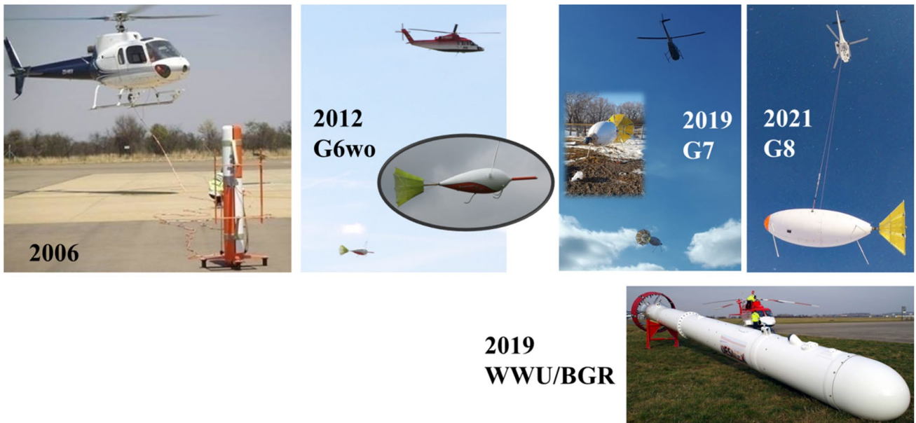
Fig. 5 The towed platforms under comparison for their motion noise. Top left is the first platform for the SQUID-based instrument which is not used for comparison due to significantly higher noise figures
